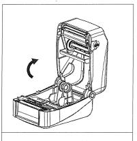
1. Press two buttons on printer two sides to lift and open the cover.
