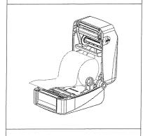
2.Load print media into the printer; adjust the paper guide to be same width of print media.
